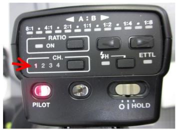
If they don't match, hold the ZOOM button until the CH. Bar blinks. Then use the large + or – buttons to change the channel until they match (all buttons and indicators marked in red below).
