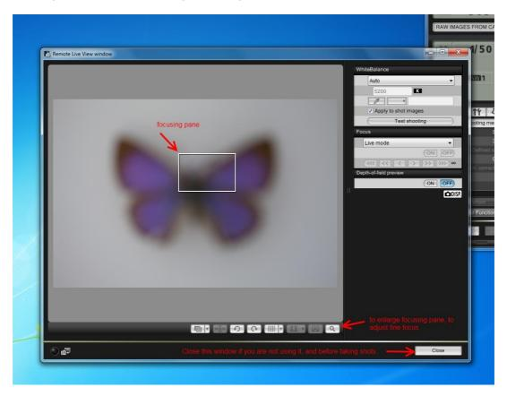
If it is two overlapping rectangles, the camera is set on automatic focus.
