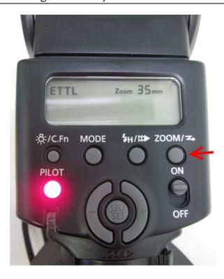
If the transmitter and flashes are still not working, check that they are on the same channel. The numbers indicated in red on the images below should match (they will always be '1').
