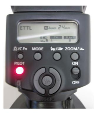
If that link has been broken, the display will look as below. Re-establish the link by holding the **ZOOM** button (marked with the red arrow) down for about 20 seconds. The flash will automatically find the transmitter and establish the relationship.
