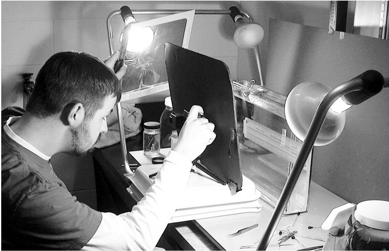
Figure 5. Kyle Luckenbill photographing small alcohol-preserved specimen (above ruler) while holding polarizing filter in lab. Photo by author.
