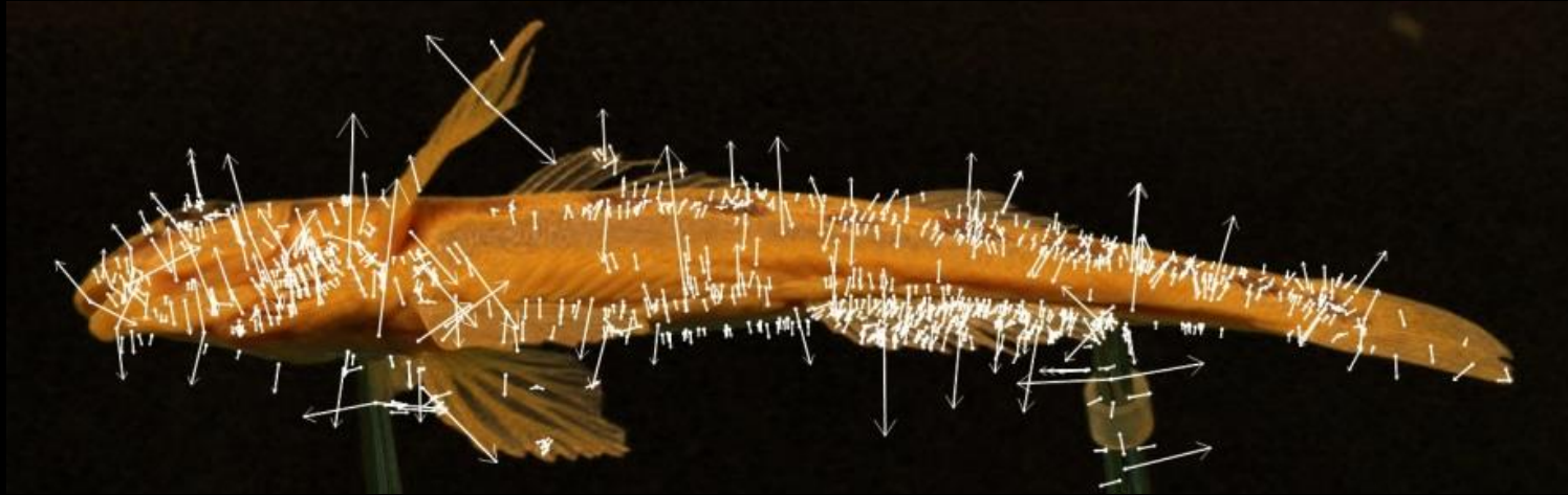
Features identified within an image using Scale Invariant Feature Transformation (SIFT). Scale and orientation indicated by arrows.
