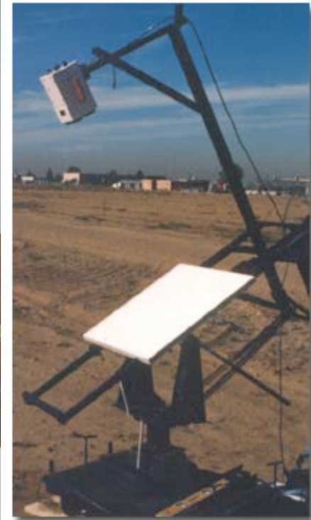
Reference Panel on Goniometer with Exotech measuring.
