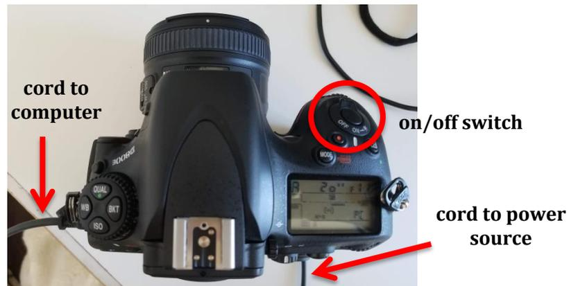
3. Turn on the computer (if necessary) and camera, in that order. The camera’s “on” switch is located to the right of the lens on the top of the camera (circled in photo above).
